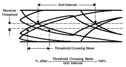
Figure 14. Measuring Signal Transmission Quality
