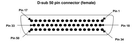
Fig. 2 D-sub 50 pin connector.
