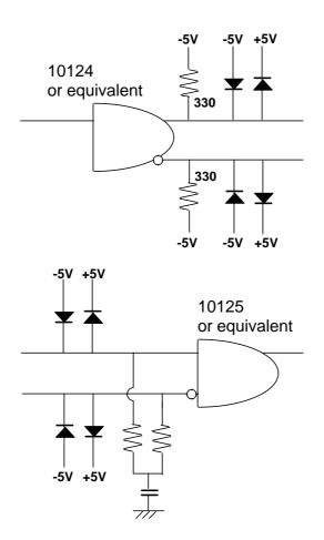
Fig. 3 ECL data transmitter and receiver with protection circuit.
