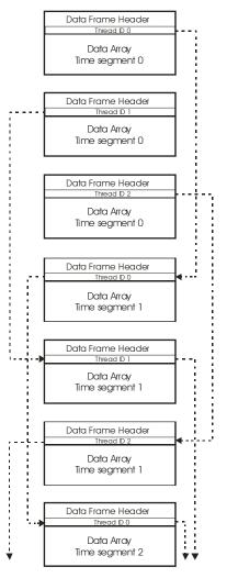
Figure 2: Illustration of Data Threads within a Data Stream
