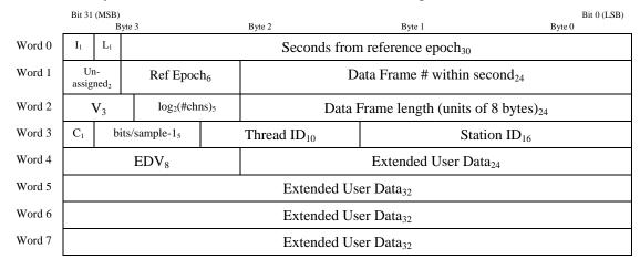
The standard 32-byte VDIF Data Frame Header is shown in Figure 3.
