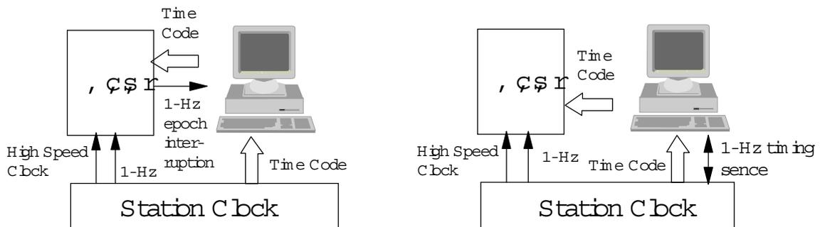
(a) Time code transfer with an interruption line    (b) Time code transfer without an interruption line
