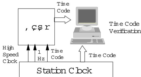
Figure 2 Hardware time code transfer
