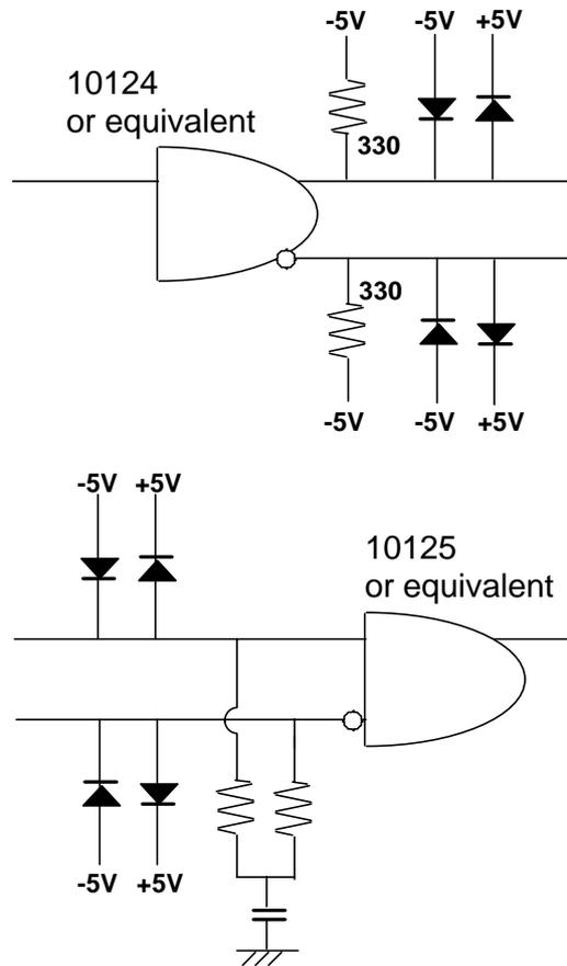
Fig. 3 ECL data transmitter and receiver with protection circuit.
