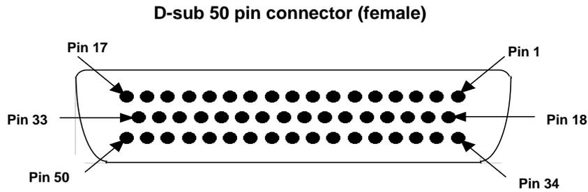
Fig. 2 D-sub 50 pin connector.
